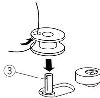
3 Pass the thread through the hole in the bobbin from the inside to the outside. Put the bobbin on the bobbin winder spindle.
