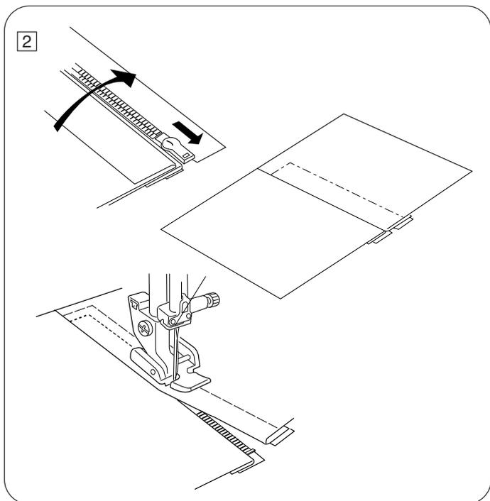
2 Raise and release foot, and re-attach it on left-hand side of pin.
