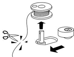
6 Start the machine again. When the bobbin is fully wound, it will stop automatically.
