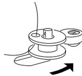
4 Push the bobbin winder spindle to the right.
