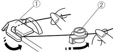
1 Hold the thread with both hands and pass the thread under the thread guide.
