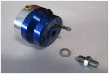
Remove adjustment screw and locking nut from the top of the Fuel Regulator. NOTE: Mark the two halves with a marker to indicate the orientation of the two halves. This way it will be clocked in the right position when put back together.
