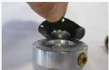
Place the diaphragm onto the bottom portion of the Regulator with the pointed end facing down.
