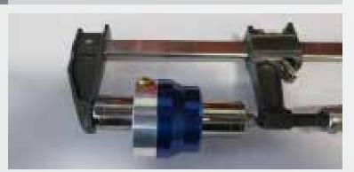
Using two 21mm sockets and a C clamp. Clamp the Fuel Regulator together firmly. NOTE: tape may be used on the two halves to prevent damage to the Fuel Regulator.
