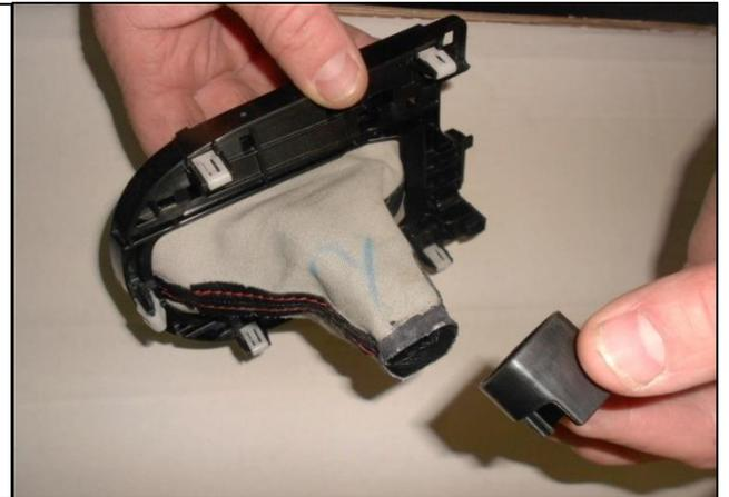
8. With the shift boot inverted, orientate the Hurst pistol grip handle in the correct position and slide it through the boot as far as it will go.
