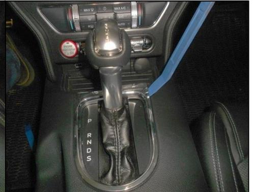
2. Starting from the front of the shift indicator, pry up to release the forward locking clips. Then work your way down the side to release the remaining ones.
