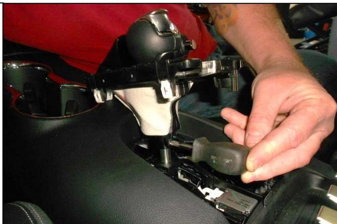
4. Remove the two Phillips screws then pull up on the shift handle to remove it.
