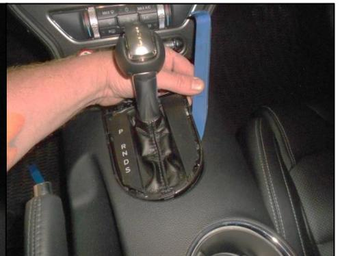
3. Raise the shift indicator high enough to unplug the wire harness from the bottom of the shift indicator.
