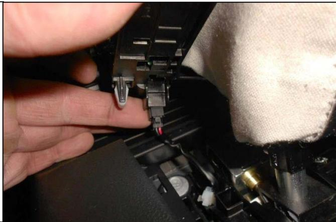
**CAUTION:** With the engine off, the emergency brake set and the front and rear wheels blocked, move the shift handle back far enough to gain access to the two Phillips screws that bolt the shift handle to the lower stick.
