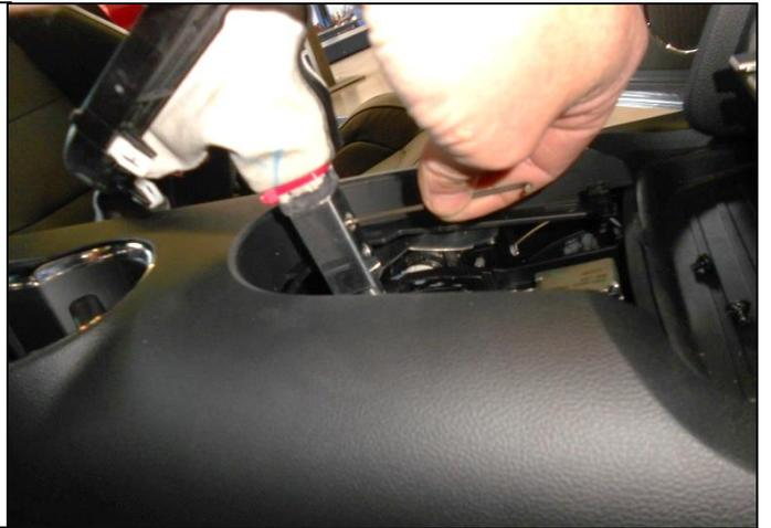
12. Put the shifter back into the Park position. Plug the wire harness back into the shift indicator and snap it back into place.
