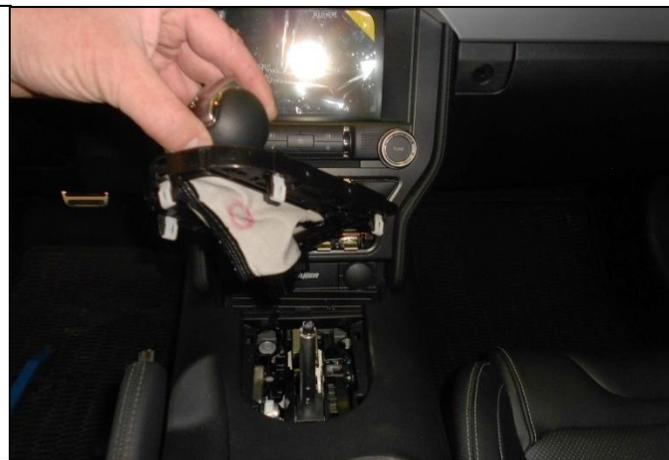
5. Release the locking tabs that secure the shift boot and gear select indicator to the shift handle.
