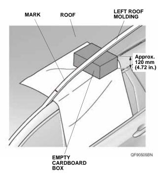
7. While wearing eye protection, use an air saw to cut the left roof molding at the mark. Do not use a cutting wheel or shears to cut the left roof molding; that can damage the left roof molding. With the help of an assistant, hold the rear edge of the left roof molding while cutting. Remove any burrs.
