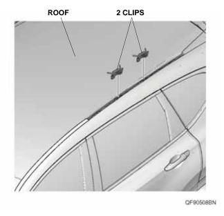
11. Using a putty knife, remove any excess sealant from the roof brackets. Apply touch-up paint to the remove sealant area, and allow the touch-up paint to dry thoroughly.
