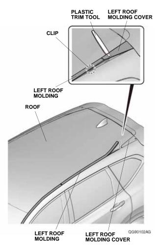
3. Remove the left roof molding from the left roof molding cover. Install the left roof molding cover.
