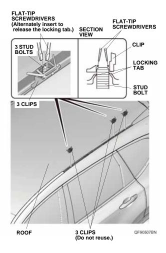
10. Remove two clips from the roof.
