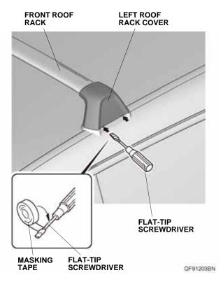
23. Remove the left roof rack cover from the left front roof rack stay.
