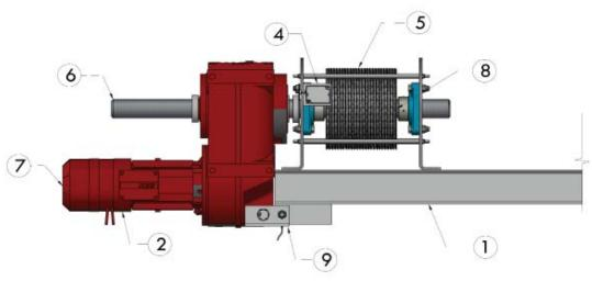
1.Frame (Backbone): The winch frame is constructed from plate steel and a "backbone" structure that can be constructed from various steel shapes. The entire perimeter of the device is to be considered the frame. The frame has a series of mounting points on the sides of the frame and along with the bottom base angles.
