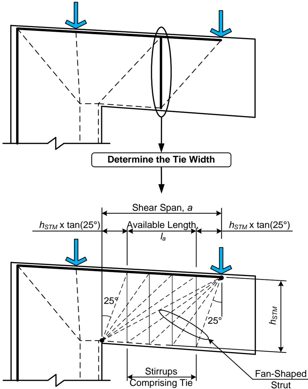
**Figure 2-13: Fan-Shaped Struts Engaging Reinforcement, Forming a Tie**
