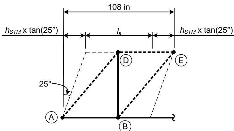
**Figure 1-10: Design Example Fan-Shaped Strut**
