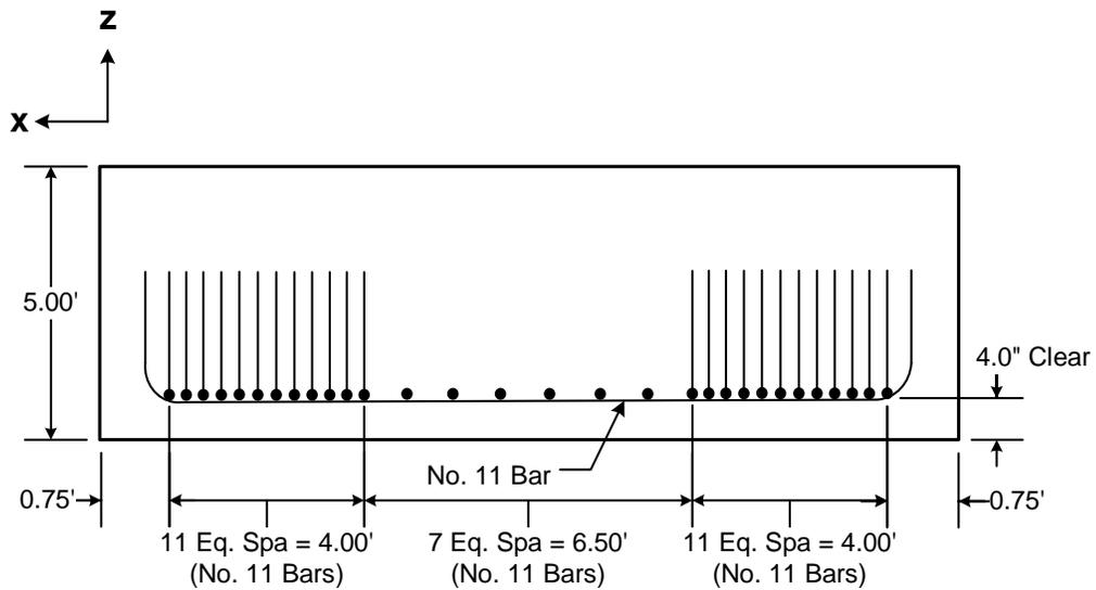
Figure 4-25: Reinforcement Details 4 - Section A-A of Figure 4-24
