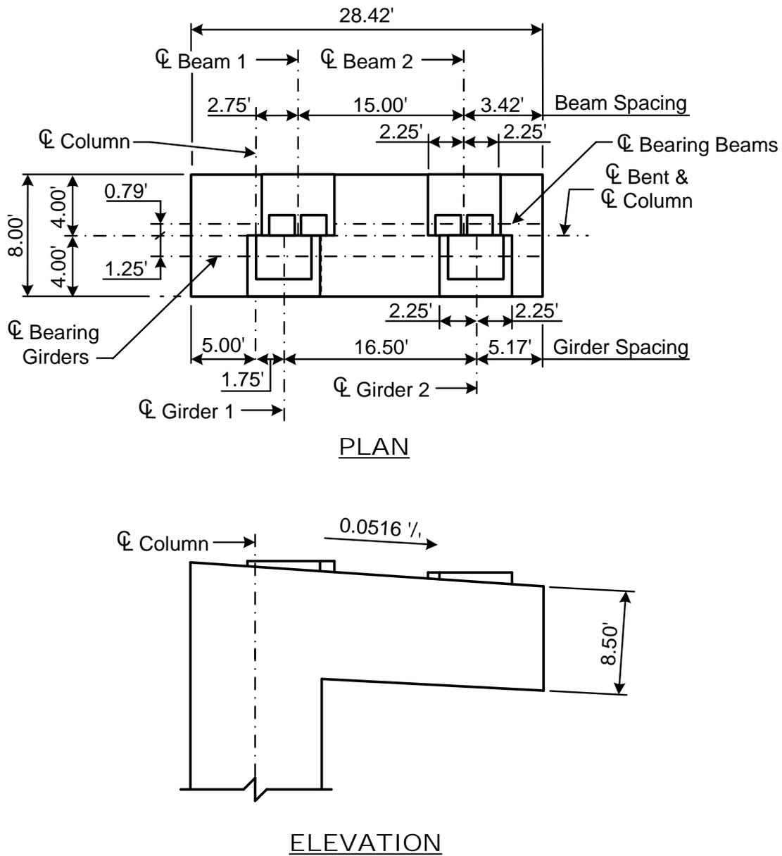
**Figure 2-2: Plan and Elevation Views of Cantilever Bent Cap (Detailed Geometry)**
