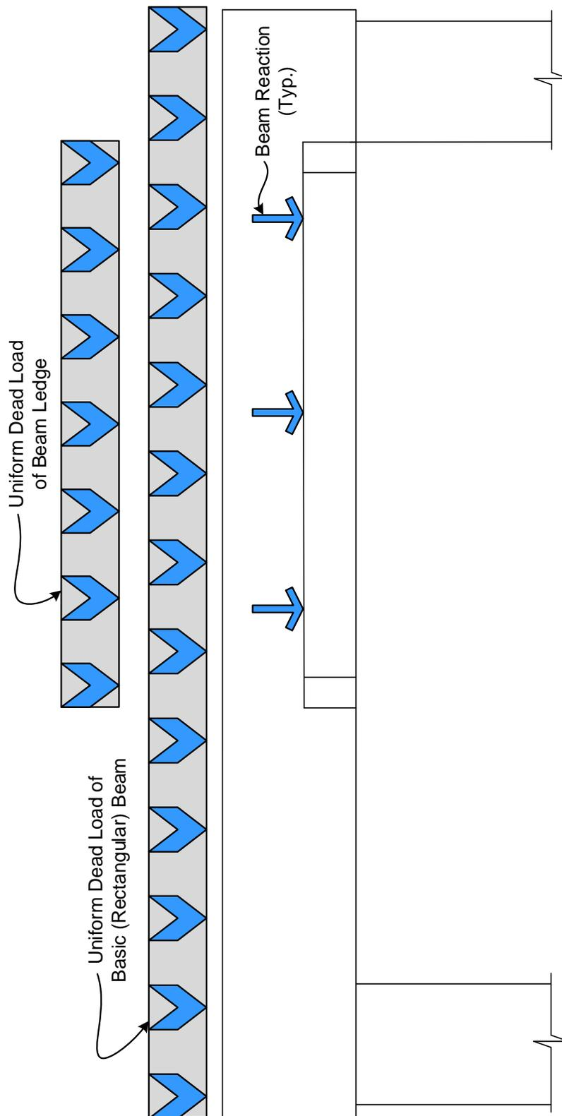
Figure 3-5: Loads Acting on the Global Strut-and-Tie Model
