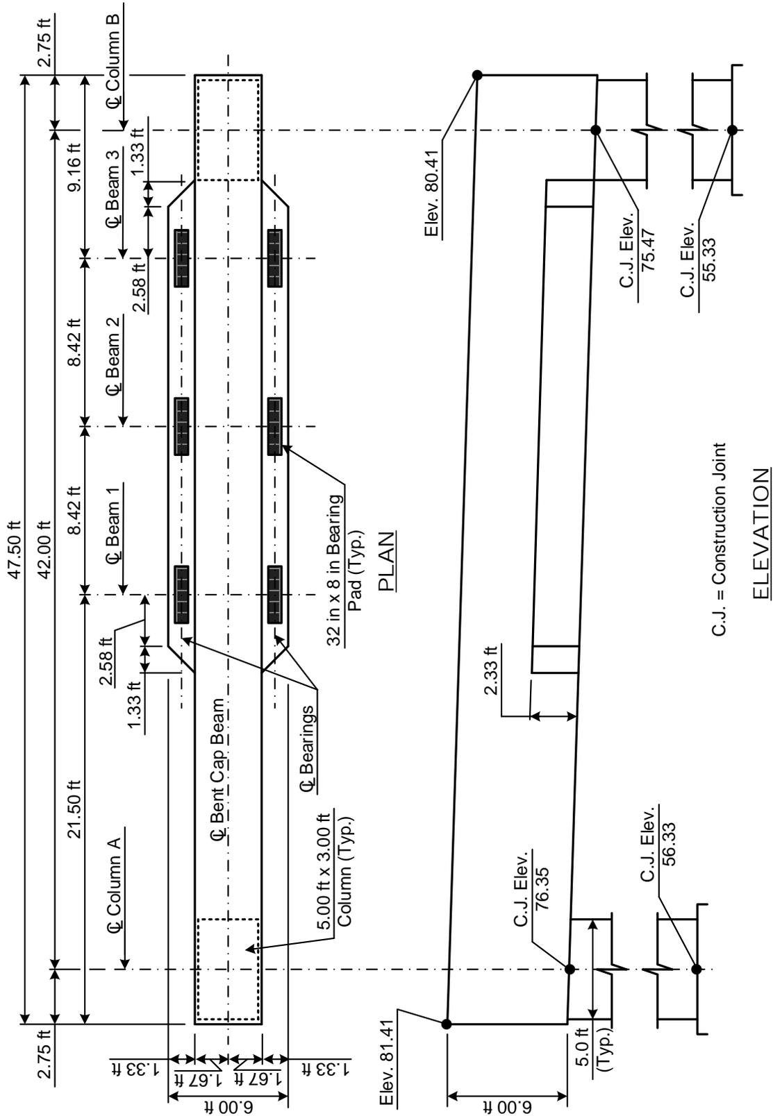
Figure 3-2: Inverted-Tee Beam Straddle Bent for Design Example 3
