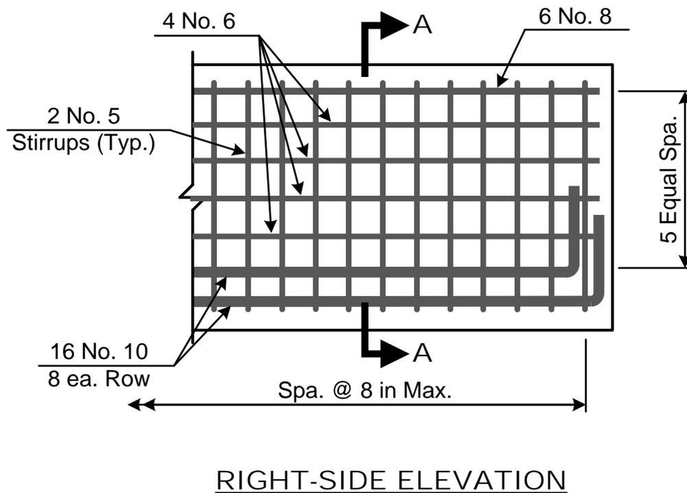
Figure 1-23: Reinforcing Layout, Right Side
