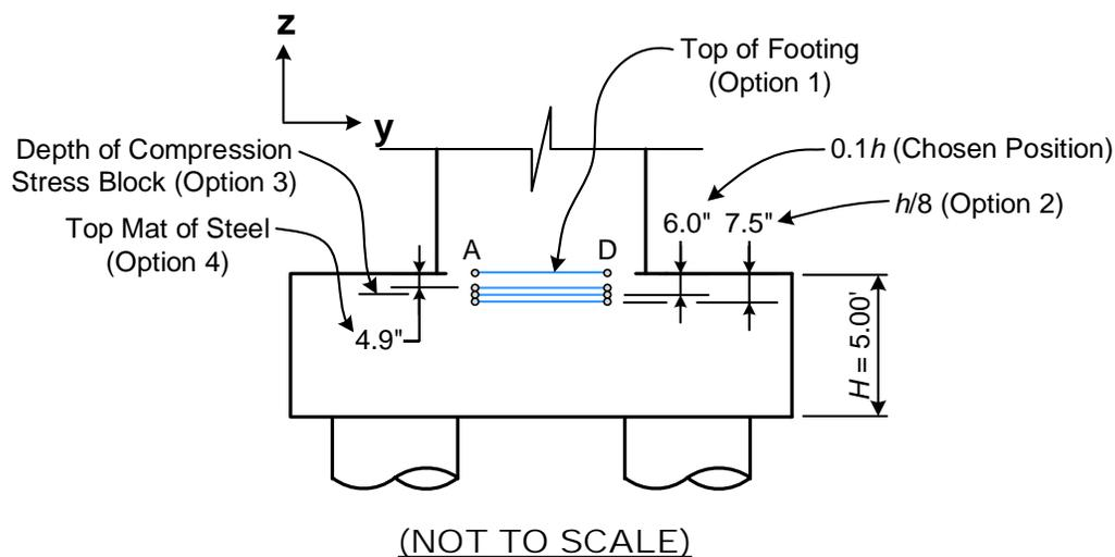
**Figure 4-10: Locations of Ties in Top of Footing**
