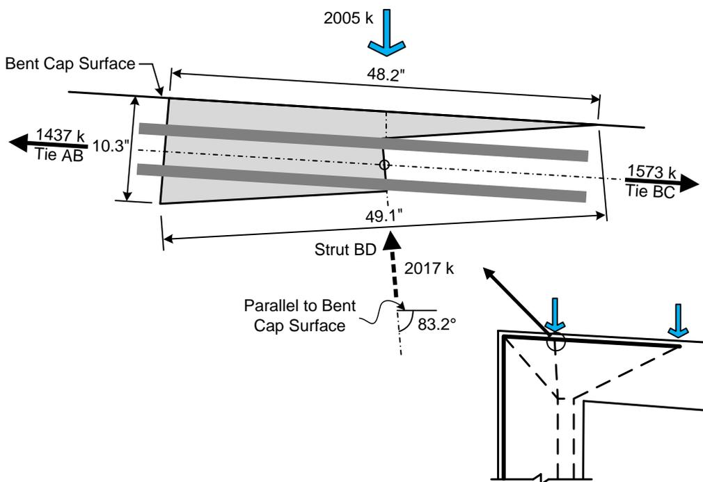
**Figure 2-15: Geometry and Forces at Node *B***
