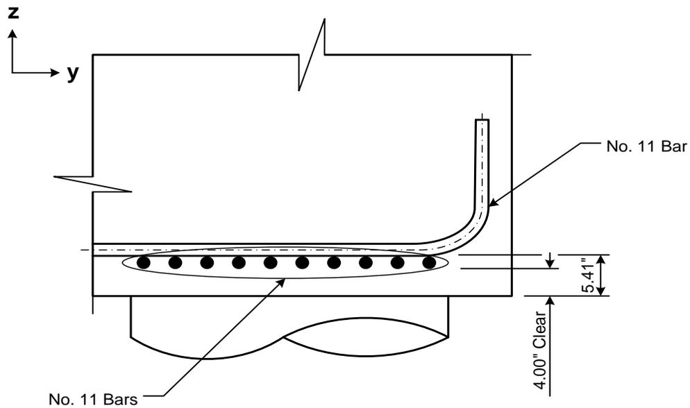
**Figure 4-7: Location of Bottom Mat of Reinforcing**
