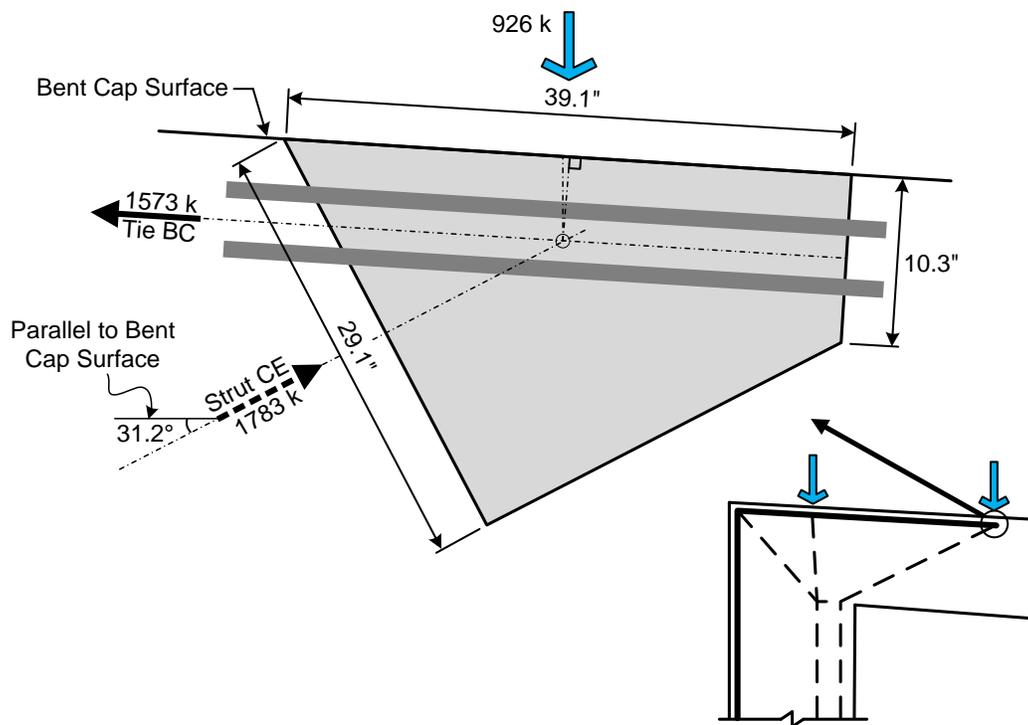
**Figure 2-16: Geometry and Forces at Node C**
