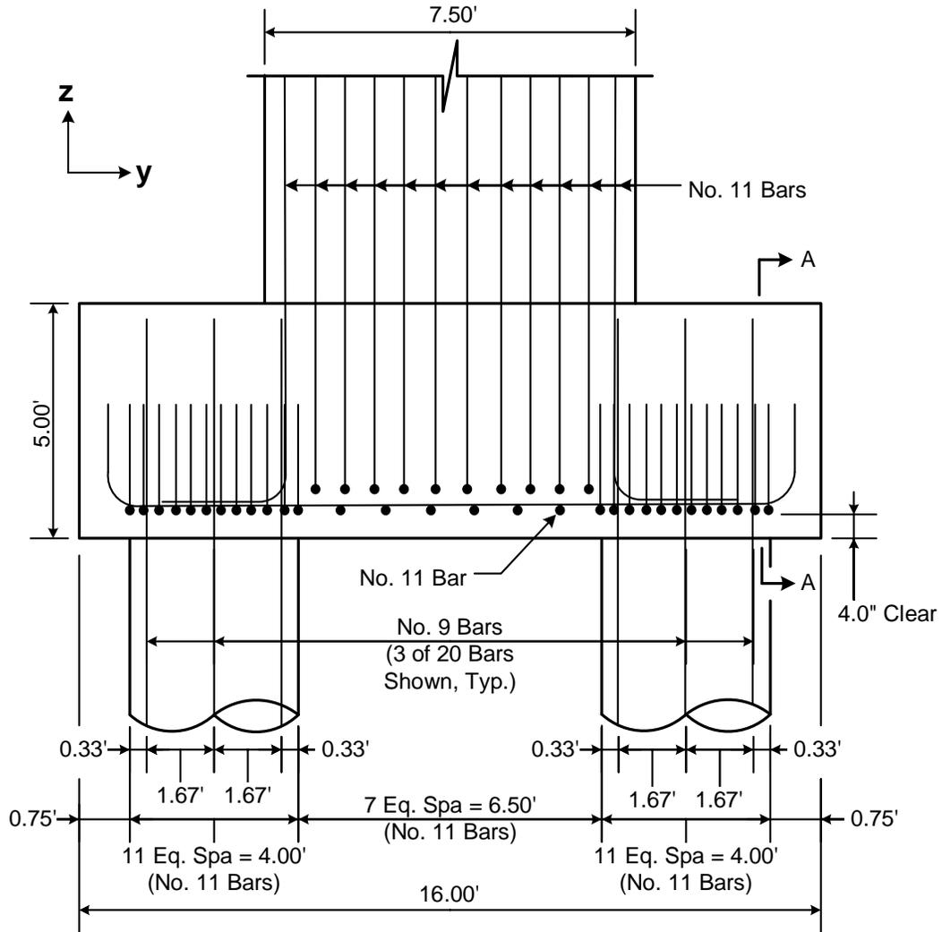
Figure 4-23: Reinforcement Details 2 - Elevation View of Primary Reinforcement
