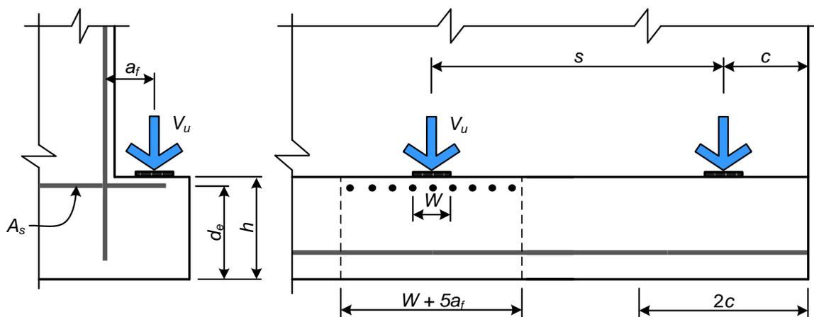
**Figure 3-18: Flexural Reinforcement for Ledges (*AASHTO LRFD* Figure 5.8.4.3.3-1)**
