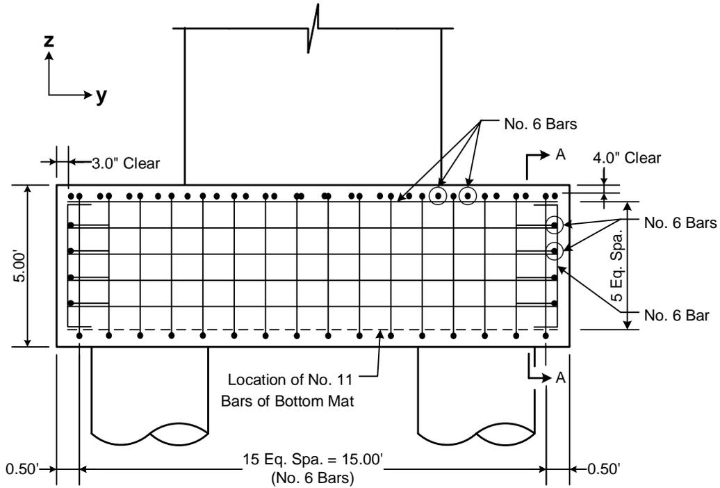
Figure 4-24: Reinforcement Details 3 - Temperature and Shrinkage Reinforcement
