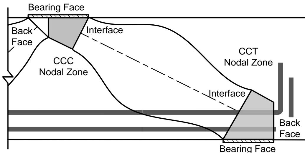
**Figure 1-5: Direct Strut-and-Tie Model of a Deep Beam**
