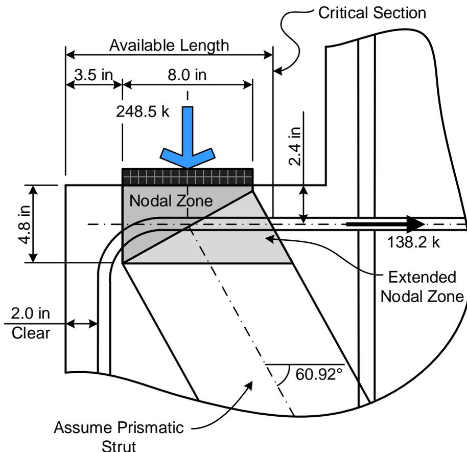
**Figure 3-28: Ledge Reinforcement Anchorage at Node  $C_s$**
