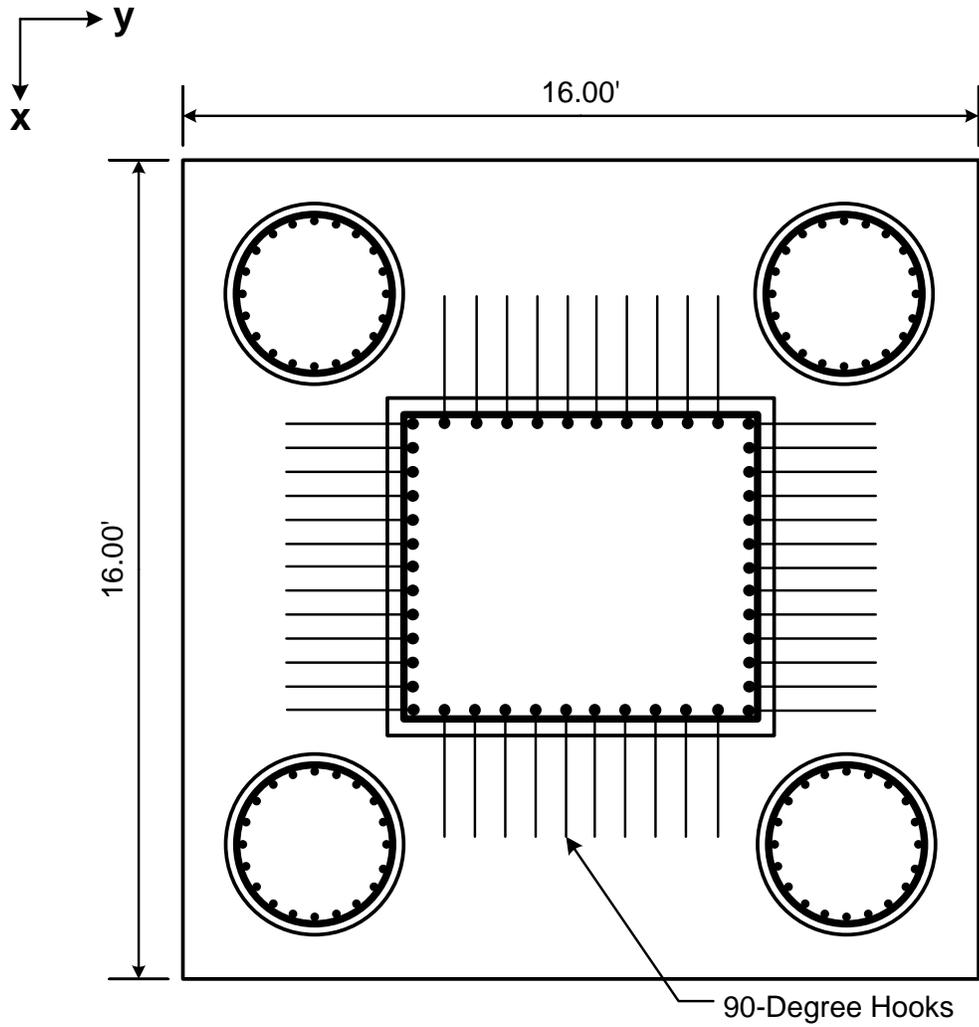
Figure 4-22: Reinforcement Details 1 - Anchorage of Ties
