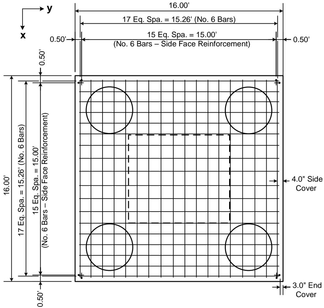
Figure 4-28: Reinforcement Details 7 - Top Mat Reinforcement
