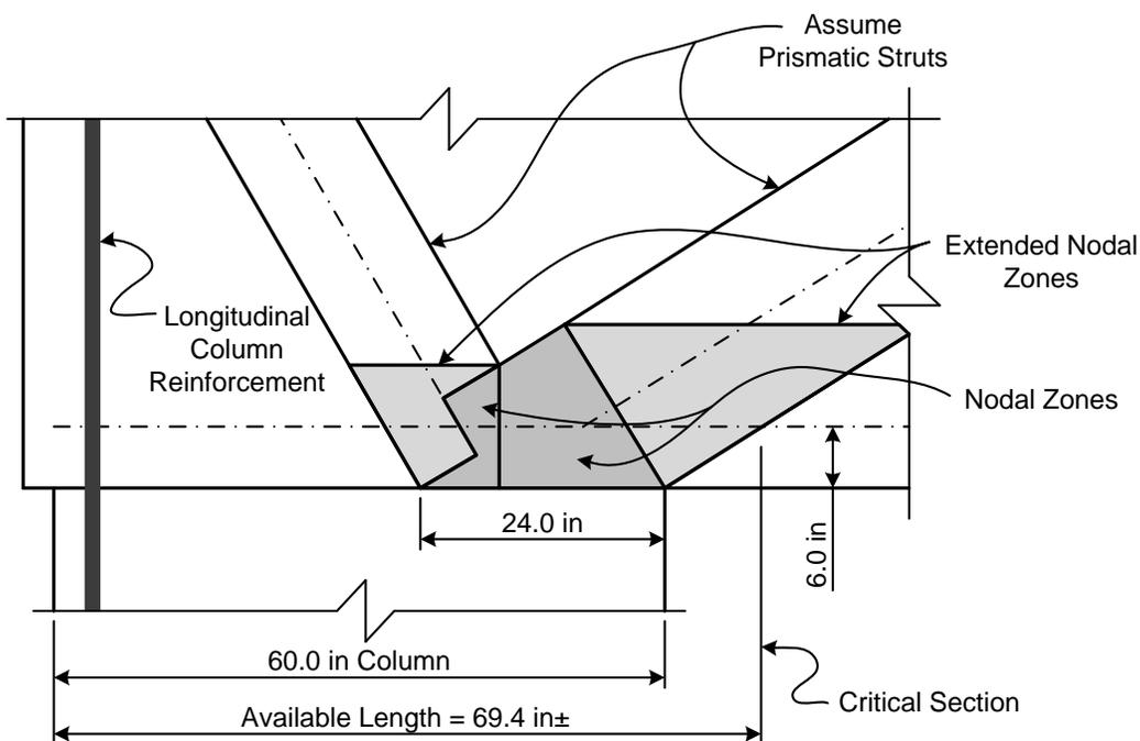
**Figure 3-27: Bottom Chord Reinforcement Anchorage at Node G**
