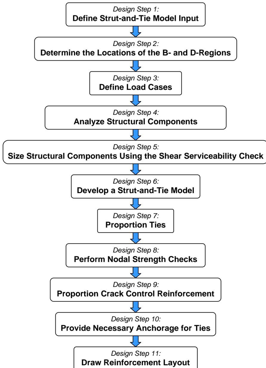
**Design Step 1 - Define Strut-and-Tie Model Input**
