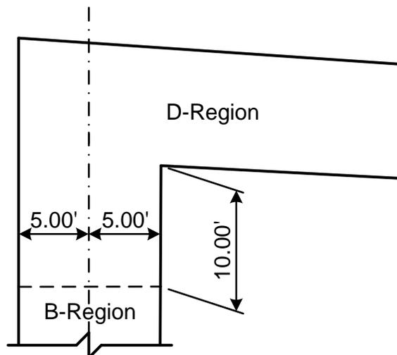
Figure 2-5: Limit of D-Region in Bent Cap
