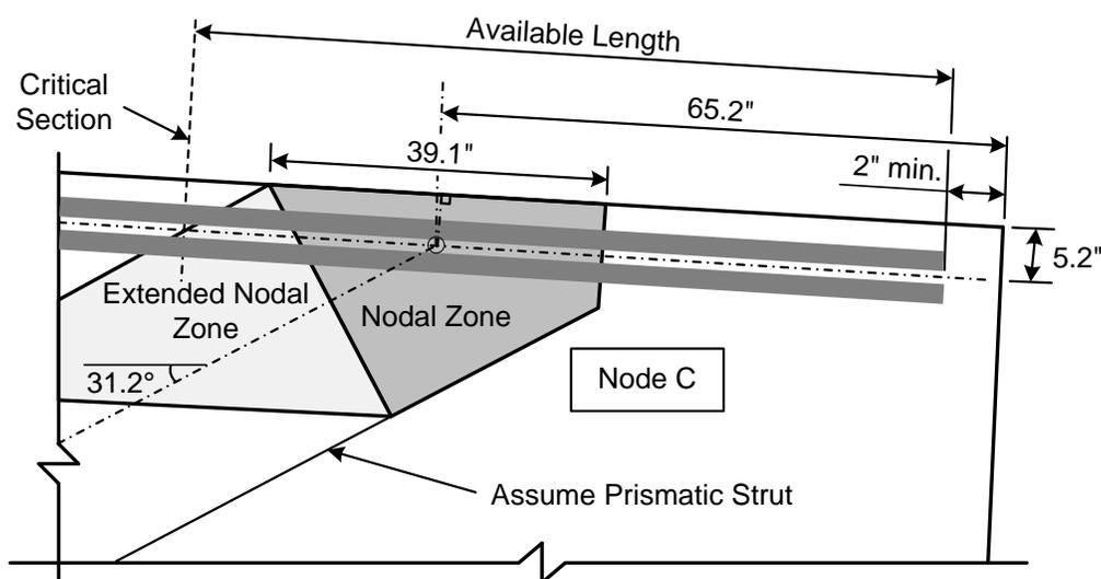
**Figure 2-17: Anchorage of Longitudinal Bars at Node C**
