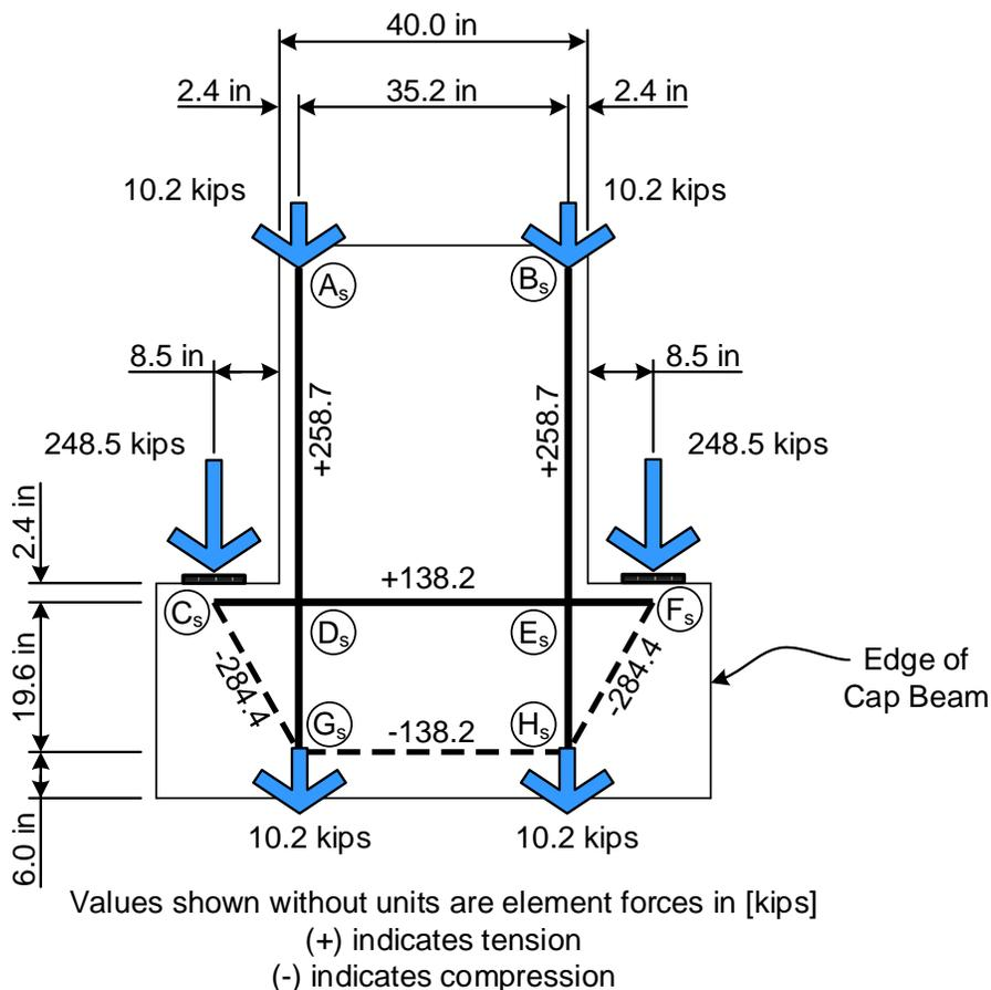
**Figure 3-11: Local Strut-and-Tie Model at Beam Line 1**
