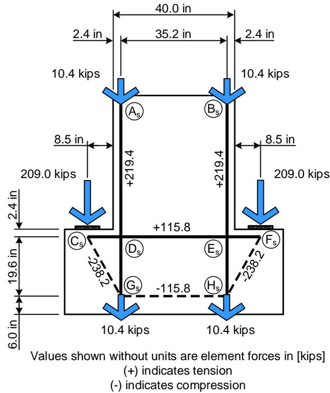
Figure 3-13: Local Strut-and-Tie Model at Beam Line 2
