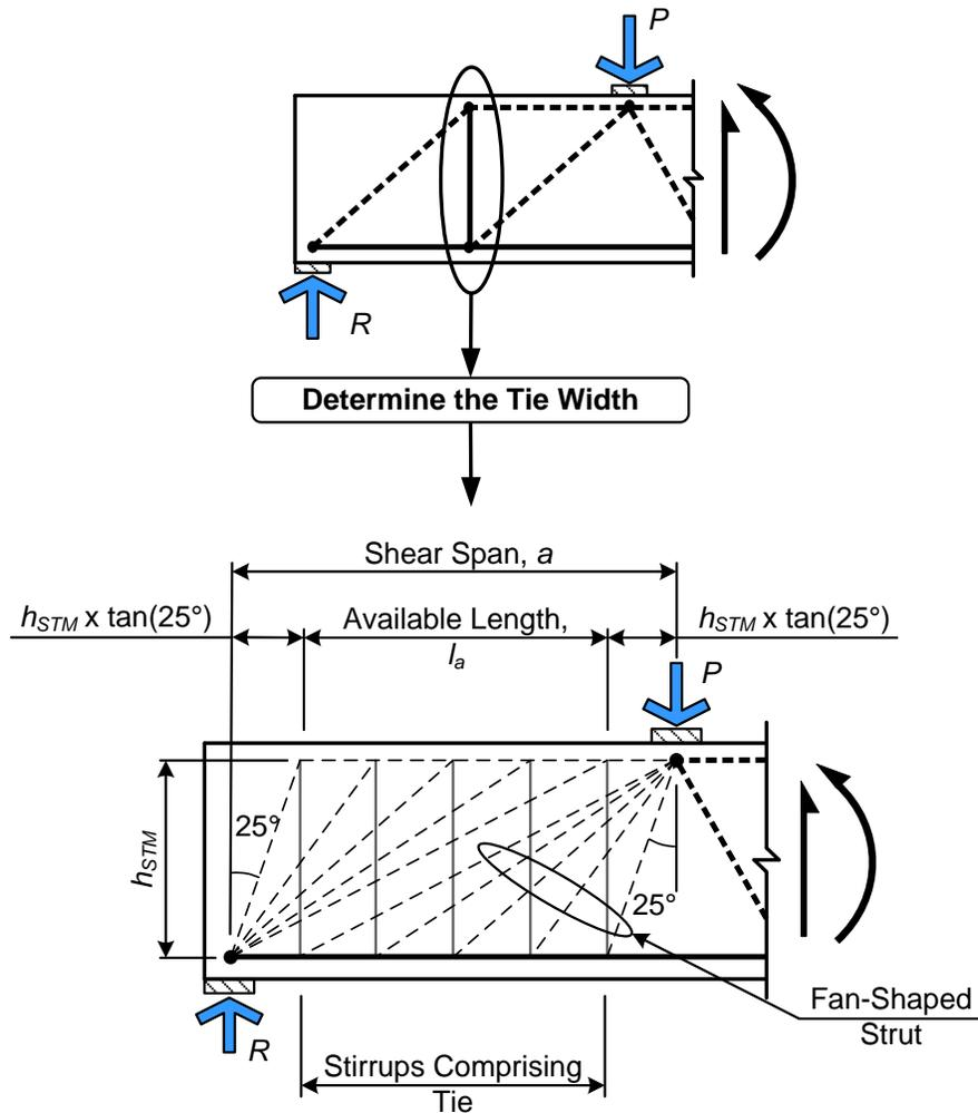
**Figure 1-9: Fan-Shaped Struts Engaging Reinforcement, Forming a Tie**
