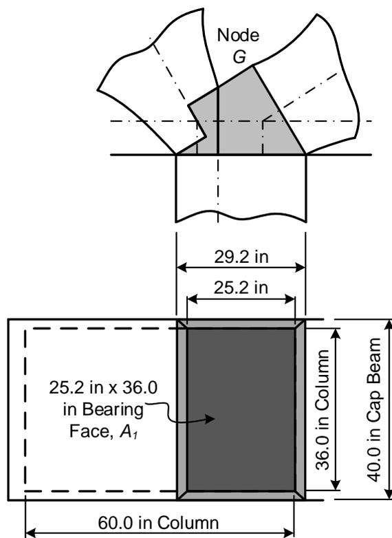
**Figure 3-22: Confinement Modification Factor,  $m$ , at Node G**
