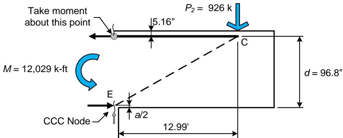
**Figure 2-12: Determining the Vertical Position of Node *E***
