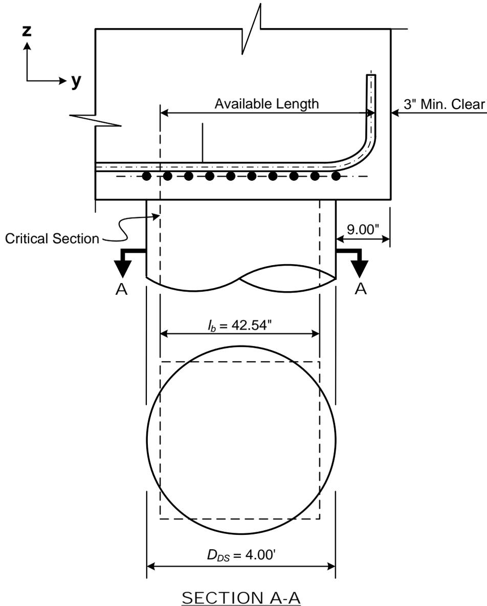
Figure 4-13: Available Development Length over the Drilled Shafts
