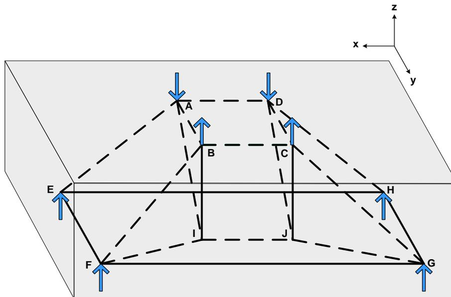
**Figure 4-11: Alternative Strut-and-Tie Model for Load Case 1**
