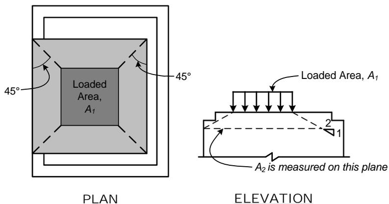
**Figure 1-14: Determining the Areas  $A_1$  and  $A_2$**
