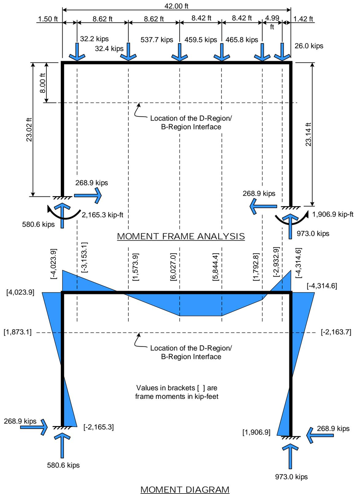
Figure 3-6: Moment Frame Analysis and Resulting Moment Diagram
