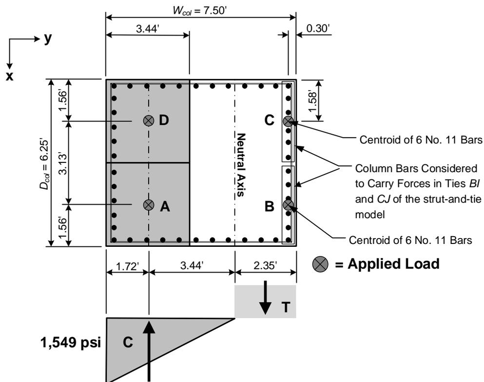
**Figure 4-6: Linear Stress Distribution over Column Cross-Section and Equivalent Force System Load Locations**
