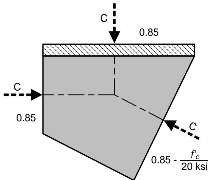
**Figure 1-17: Concrete Efficiency Factors for CCC Nodes**
