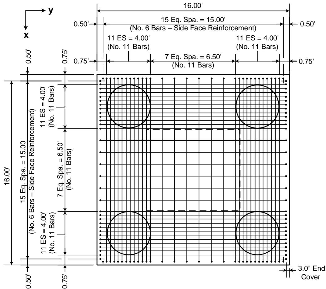
**Figure 4-27: Reinforcement Details 6 - Bottom Mat Reinforcement**
