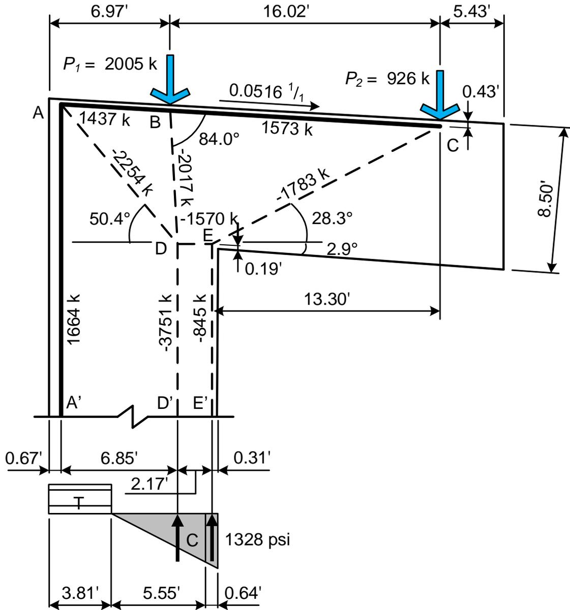
Figure 2-9: Strut-and-Tie Model Featuring One Truss Panel for the Cantilever Bent Cap
