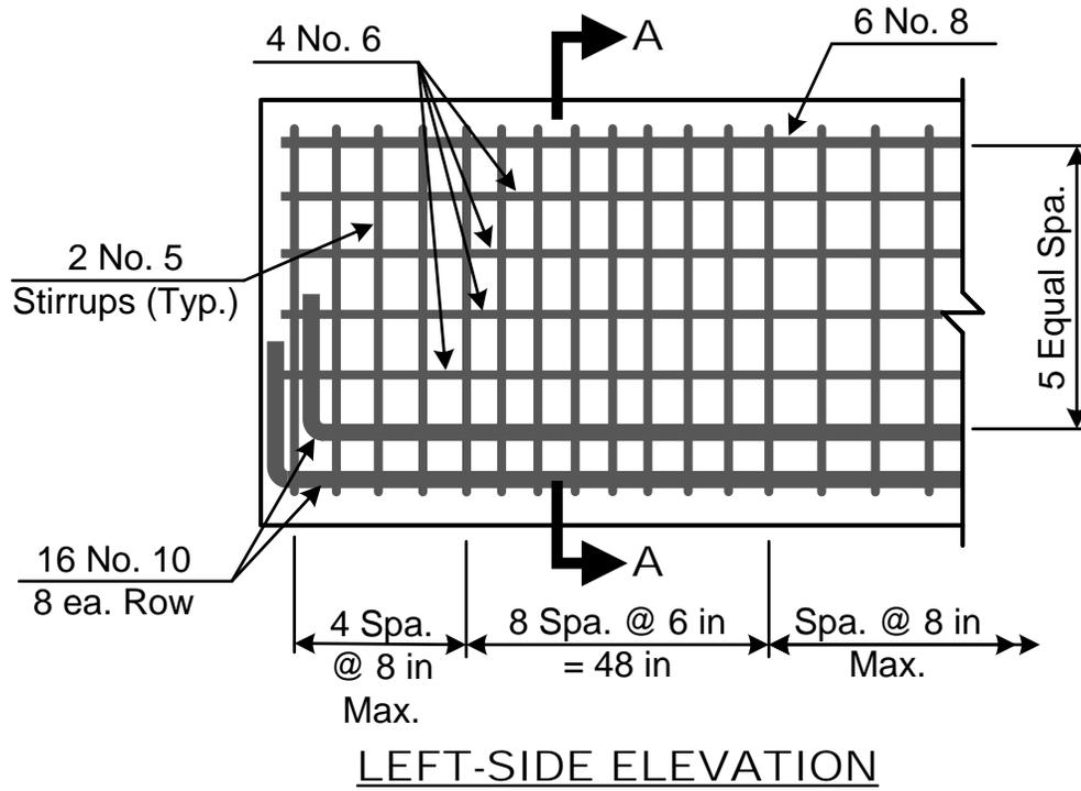
Figure 1-22: Reinforcing Layout, Left Side
