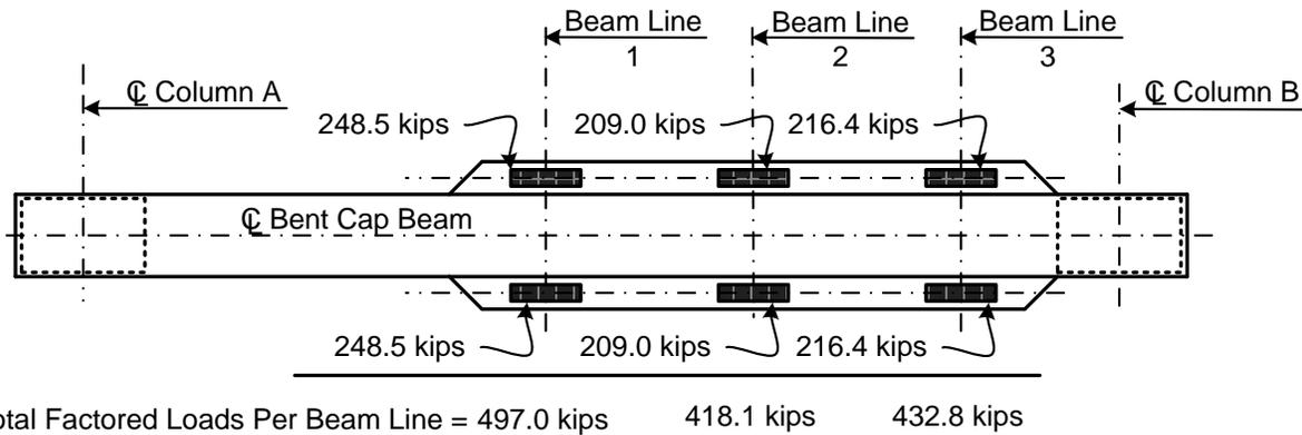
**Figure 3-4: Factored Beam Loads per Beam Line**
