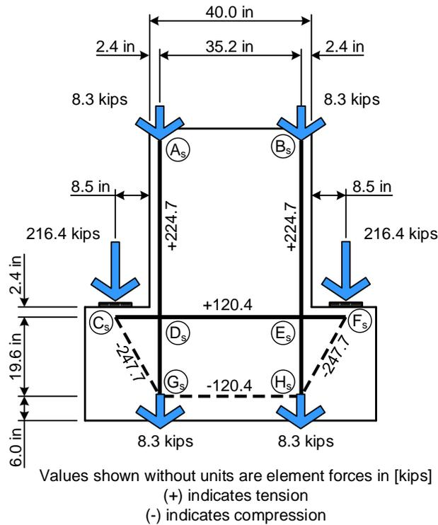
Figure 3-14: Local Strut-and-Tie Model at Beam Line 3
