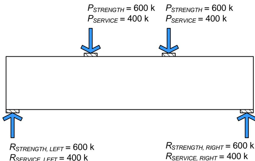
**Figure 1-3: Beam Applied Loads and Reactions**
