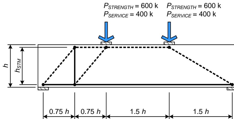
**Figure 1-7: Example Beam and Trial Strut-and-Tie Layout**
