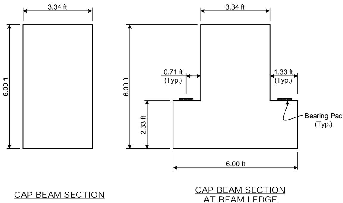
**Figure 3-1: Typical Sections of Straddle Bent Cap Beam**
