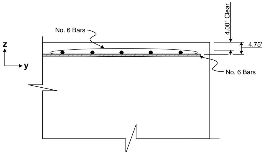
**Figure 4-17: Locating Top Mat of Footing Reinforcement**
