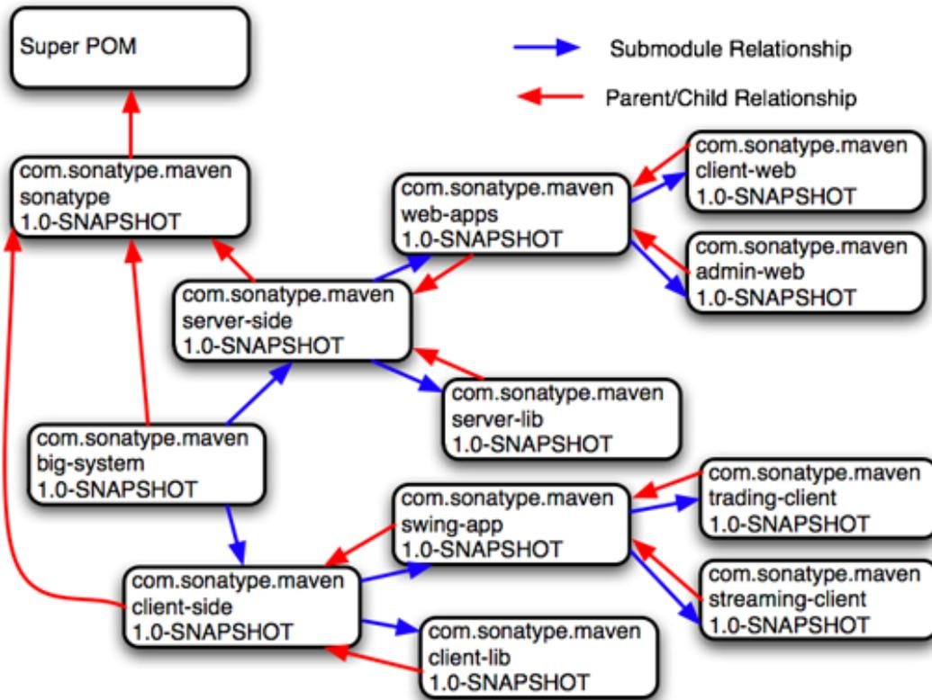
Figure 3.5: Enterprise Multi-module vs. Inheritance
