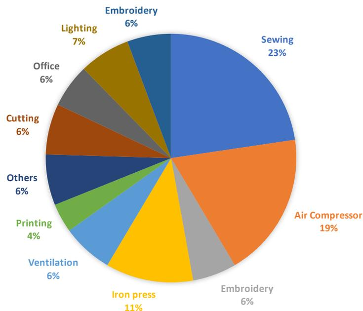
Figure 2-1 Energy consumption in the Apparel Industry
