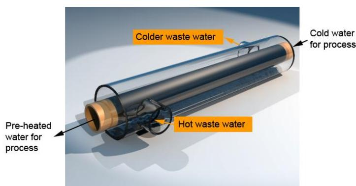
Figure 8-1 Hot water recovery systems at preheating
