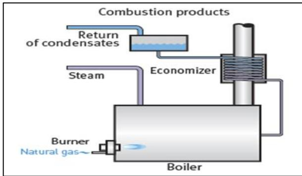
Figure 8-3 Economizer for boiler waste heat recovery
