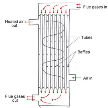
Figure 8-2 Waste heat recovery from boiler flue gas
